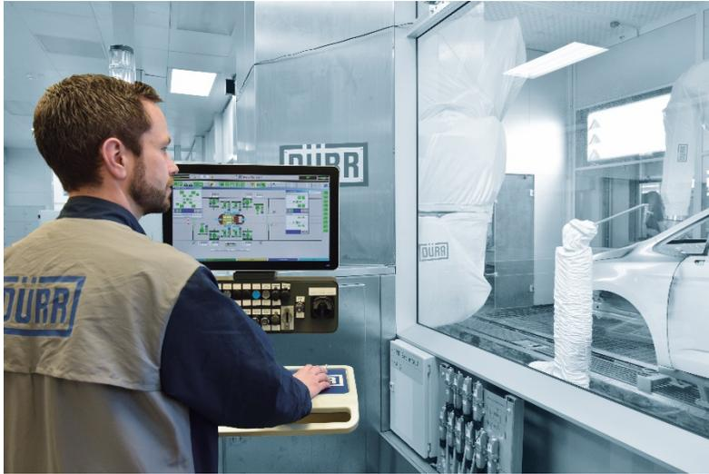
*With the new Equipment Analytics software, the plant operator can monitor the condition in the painting cell.*
